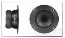
This High end cone tweeter uses a strong magnet structure for high efficiency. The ferrofluid cooled Kapton former voice coil ensures good power handling capacity. The phase plug equalizes the high frequencies. Easily coupled with 2nd order crossover as shown Fig 1. Two crossover points are suggested for adequate power handling.
