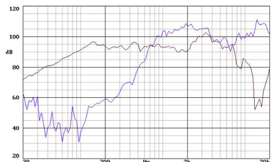
Note: on axis frequency response of low and high frequency units, 1w @ 1m.
