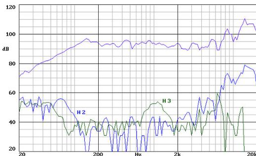
Note: on axis filtered frequency response measured with loudspeaker standing on infinite baffle in anechoic chamber, 1w @ 1m.
