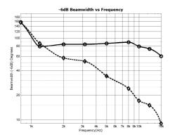
There is also an important improvement in the directivity pattern; its constant directivity characteristics ensure the ability to cover 80° wide horizontally and 30° wide vertically at virtually any frequency within its operational range.
