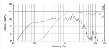
FREQUENCY RESPONSE MADE IN 125 LT. ENCLOSURE TUNED AT 50 Hz IN FREE FIELD (4n) ENVIRONMENT. ENCLOSURE CLOSES THE REAR OF THE DRIVER, THE THIN LINE REPRESENTS HIGH FREQUENCY RESPONSE FREE AIR IMPEDANCE MAGNITUDE CURVE
