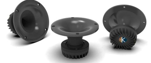
Compression driver with low compression rate through the phase plug and direct front radiation. The back cover is designed to cool the voice coil through the motor structure. It reproduces 3000Hz to 25000Hz with extreme linearity, and very low distortion.
