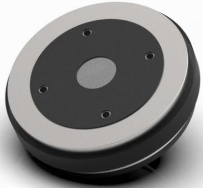
Cmp50\_vPA-S is a compression driver dedicated to high quality monitoring systems (typically high efficiency, 2 ways). The motor structure uses a 134mm diameter Ferrite magnet (grade Y40), optimized pole pieces design made of low carbon steel, and it is demodulated by Aluminum ring. The diaphragm is made of treated Titanium and very light Aluminum voice coil wired on Polyimide former. It has been engineered to provide dynamic and accurate sounding with very low THD from 1kHz to 20kHz.
