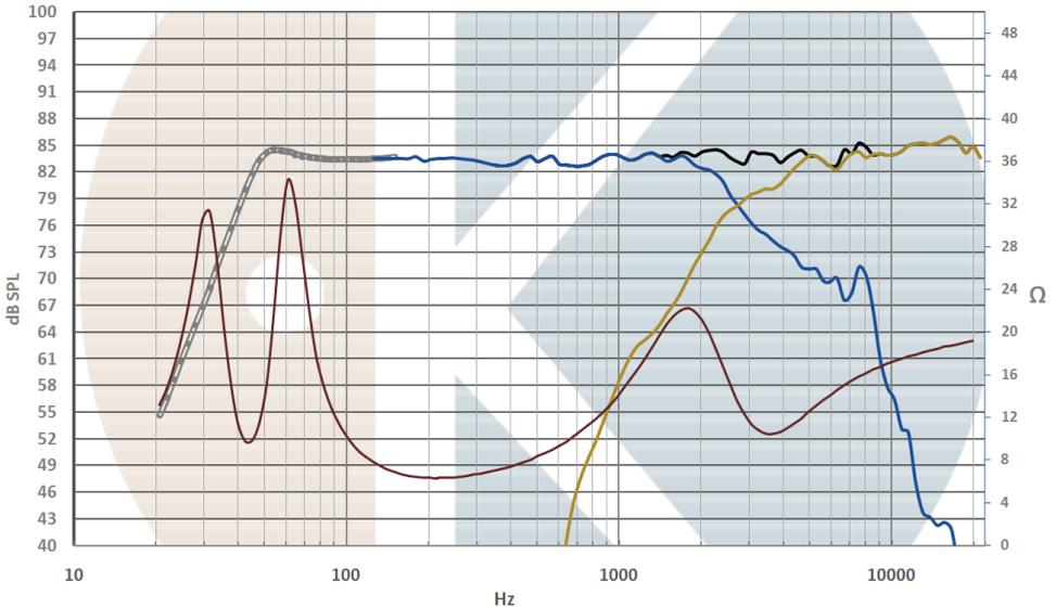
*Kourtisane 4.2 / Distance: 1m / Signal input: 2,83V / On axis
