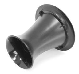
Vent with optimized cross section to avoid noises and turbulences in the air flow. It is quiet with air speed until 22m/s.
