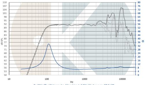
On IEC baffle / Distance: 1m / Signal input: 2,83V / Dash curves: 30° & 60° Impedance measured in free air / Smoothing: 1/12 Octave Curve below 180Hz is simulated in 1.25L Sealed enclosure, Fc = 195Hz, Qtc = 0.75
