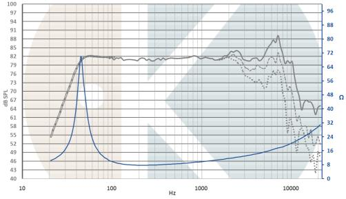
On IEC baffle / Distance: 1m / Signal input: 2,83V / Dash curves: 30° & 60° Impedance measured in free air / Smoothing: 1/12 Octave Curve below 100Hz is simulated in 5.5L vented enclosure, Fc = 45Hz
