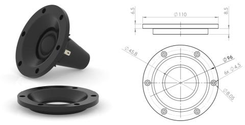
This horn provides higher sensitivity to the Twt30\_vMS in the mid-band. As a consequence, the Twt30\_vMS can play higher sound level with very low THD, or reach soft crossover point around 1800Hz.
