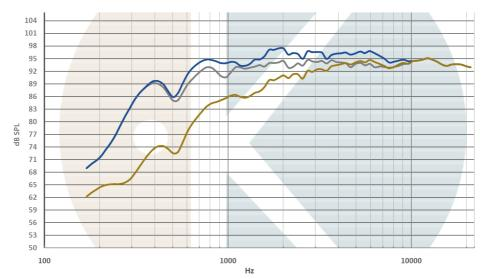
On IEC baffle / Distance: 1m / Signal input: 2,83V Grey: Twt30\_vMS / Blue: With Horn-30 / Orange: With Horn-30 + 5,6µF capacitor
