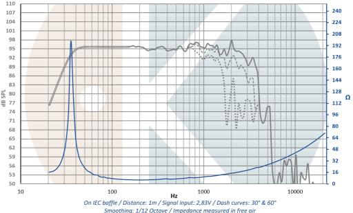
Curve below 150Hz is simulated in 150L vented enclosure. Fc = 35Hz
