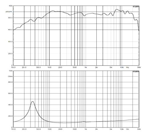
FS 34.2417 Hz **VAS** 58.8923 L RE  $7.2000 \Omega$ QMS 2.3823 0.4411 **QES QTS** 0.3722 SPL 89.3145 SD 0.0147 m2 1.9409 mm/N **CMS MMS** 11.1310 g RMS 1.0052 WM MMD 10.1179 g ZMIN 7.9869 W ZMAX 46.0862 W L1kHz 0.1272 mH L10kHz0.0907 mH X Max 9mm (1 way) Pwr 50 Watts (Nom)
