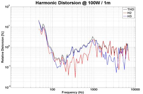
Non linear curves measured thanks to Klippel software and hardware, in free air
