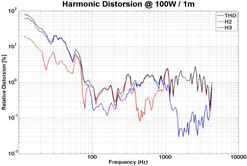
HD curves measured on CEI standard baffle : . at 1 meter . at power = P\_AES / 4
