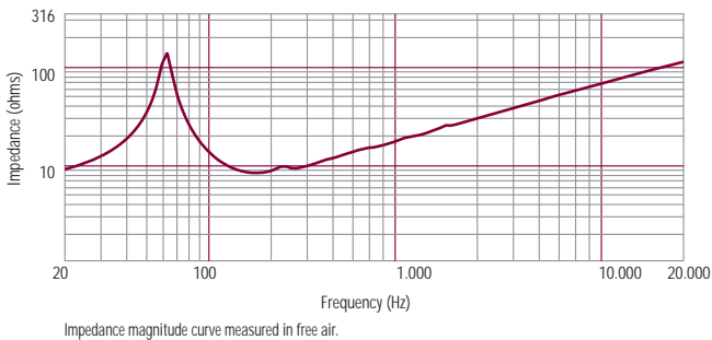
Impedance magnitude curve measured in free air.
