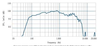
Frequency response curve of the loudspeaker made in a hemispherical, free field and mounted in a reflex box with an internal volume of 50 litres and tuned at 60Hz, applying a sinusoidal signal of  $2.83\,V@8$  at 1m.
