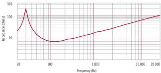
Impedance magnitude curve measured in free air.
