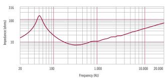
Impedance magnitude curve measured in free air.
