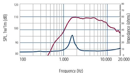
Frequency response curve of the horn measured on axis at distance of 1 meter with 1 watt signal, in an anechoic environment, with ND1411-M compression driver.
