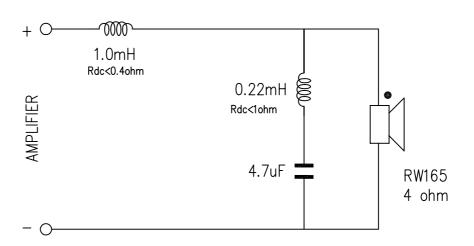
Capacitor must be Polypropylene foil type, 160V rating
