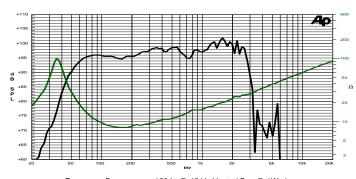
Frequency Response on 150 Lt @ 45 Hz Vented Box @ 1W, 1m Free Air Impedance
