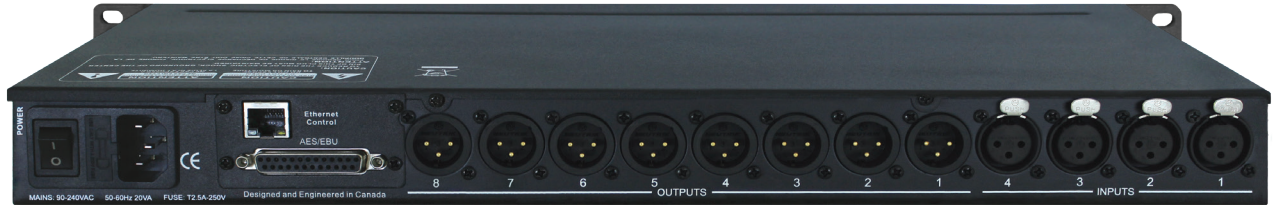
Above: Rear panel view of the XD-4080, with XLR I/O section.
